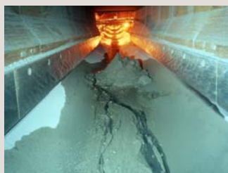
HARDOX 600 as lining in mineral transporters.
