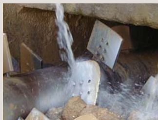
HARDOX 600 in log(stone) washing paddles.
