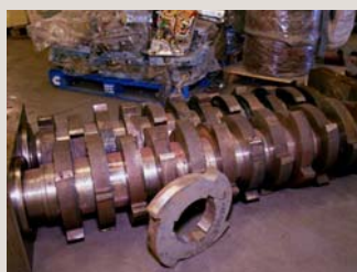
HARDOX 600 in shredder knives.
