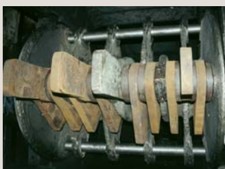
HARDOX 600 in hammers for waste fragmentation and recycling.
