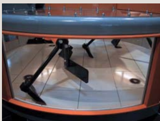
HARDOX 600 as linings in concrete mixer.
