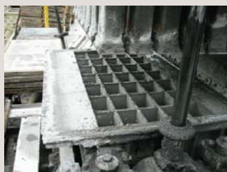
HARDOX 600 in concrete brick mould, table and compactors.
